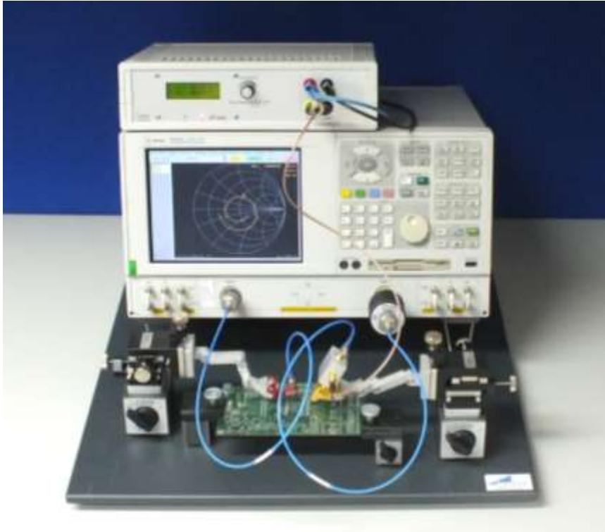
Figure 3: the new eFuse 3-080-30 together with the MAPS probe station [2] for boards
